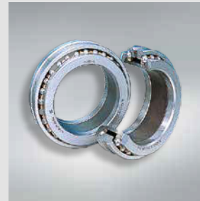
Double Row Angular Contact Thrust Ball Bearings NSKTAC D Series 60° contact angle with the highest axial rigidity. Separable type.
